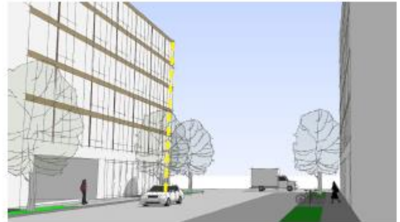
Figure 19: Street without upper-level setbacks
