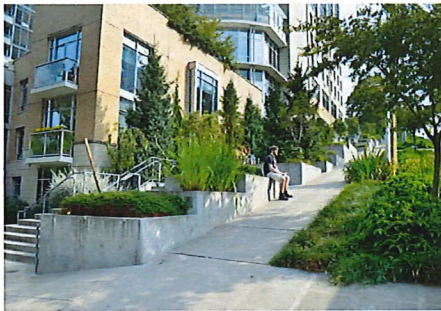
Accessibility of a sloping sidewalk is enhanced by resting spots and stair with handrails.
