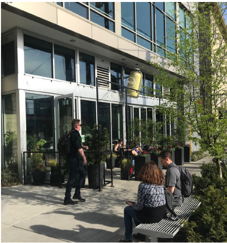
An angled building setback, operable storefront, and space for cafe seating along the sidewalk is complemented with public benches built into the sidewalk planting strip.
