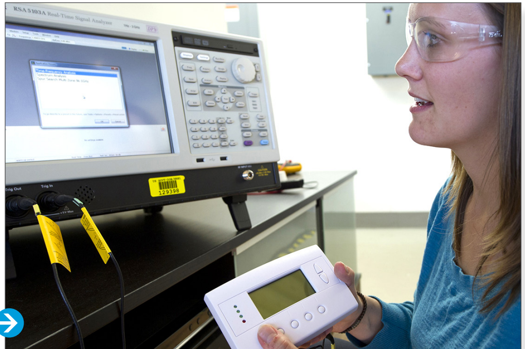
Engineer Bethany Sparr measures energy consumption at NREL's Automated Home Energy Laboratory which allows researchers to study the complex interactions of multiple appliances and devices with the broader distribution grid. Photo by Dennis Schroeder, NREL 20164.
