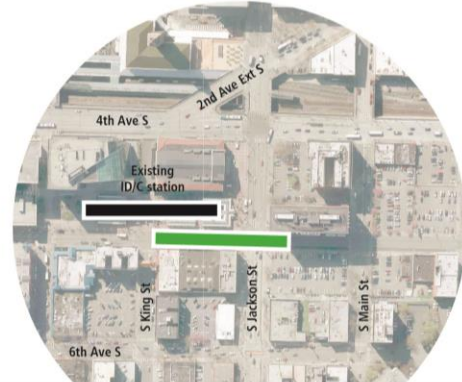
Station location alternative (straddle S Jackson St) Note: applicable to both cut and cover and bored tunnel alternatives
