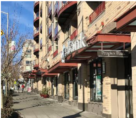
Avoid deeply recessed windows at street level that lack individuality, and do not encourage interaction between shops and pedestrians.
