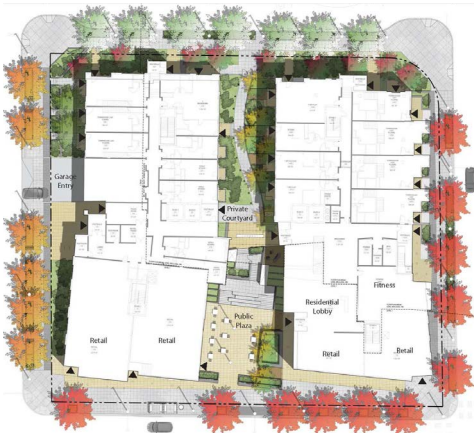
Example of massing of building broken to allow for sunlight, natural ventilation, and plaza space.
