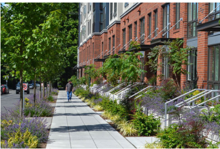
Ground-level setback zone with residential patios and wide planting strips with new shade trees
