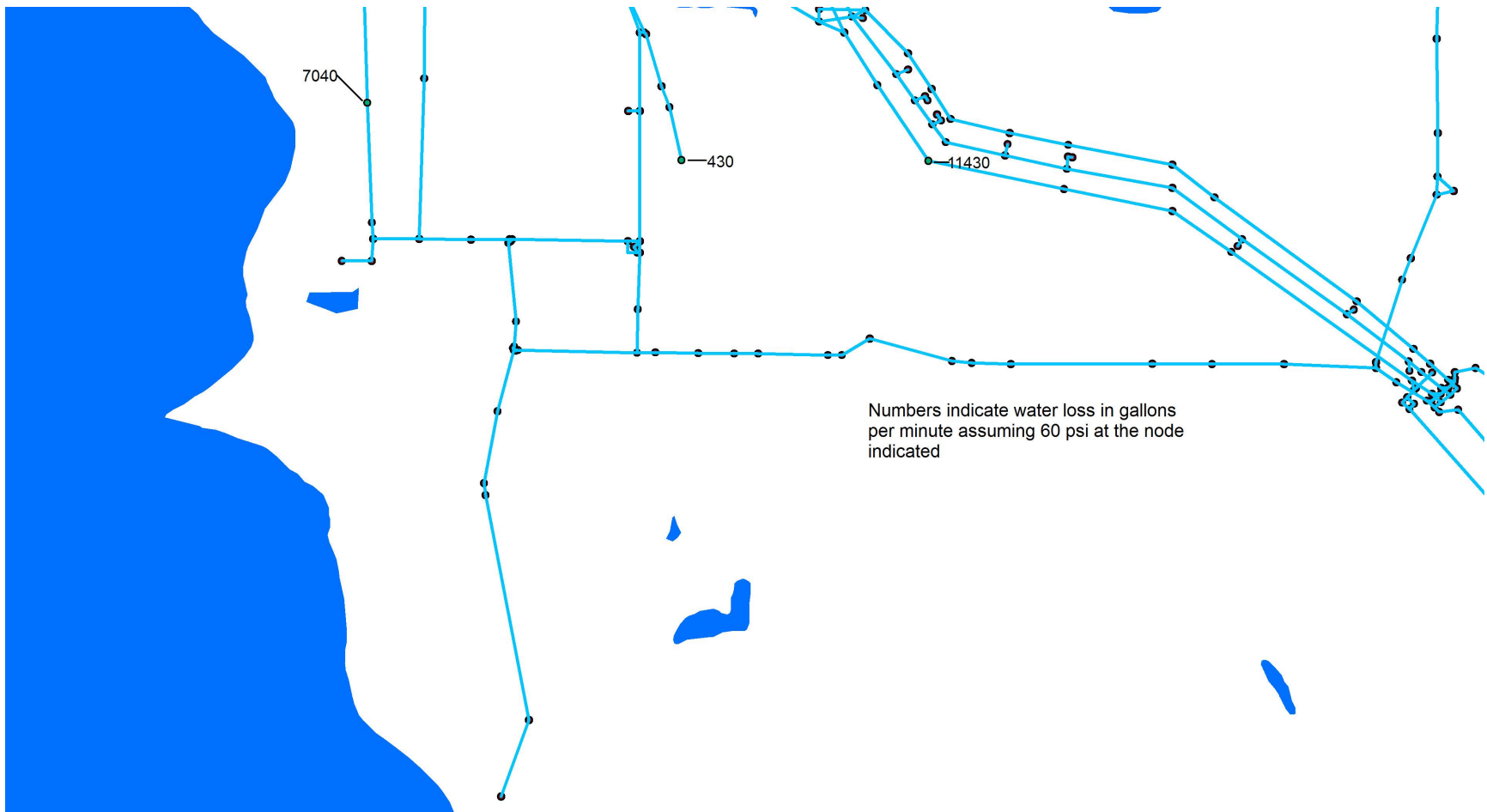
Figure 5-5. Water loss (gpm) at 60 psi for M7.0 SFZ scenario (southern direct service area)
