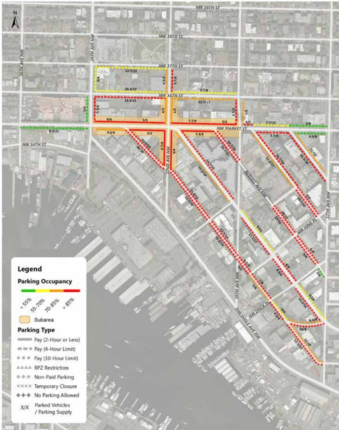
Figure 8: Ballard On-Street Parking Occupancy, Average Peak 3 Hours of each blockface during 8AM-5PM, Source: http://www.seattle.gov/transportation/parking/docs/SDOT2014ParkingMaps.pdf , 2014
