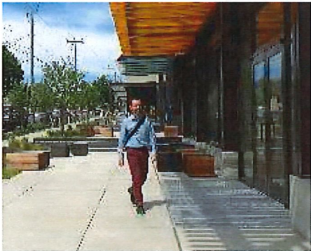
Where street slopes, establish a flat grade at the main entry and use a setback to adjust the grade against the building and provide full-height windows.
