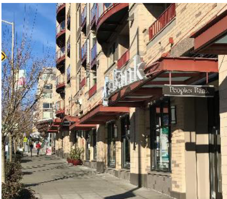
Avoid deeply recessed windows at street level, as shown above, that lack individuality, and do not encourage interaction between shops and pedestrians.
