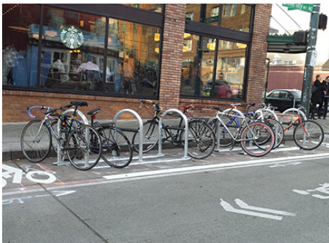
A bike corral with “inverted U” style racks provide ample and convenient parking without blocking sidewalks.
