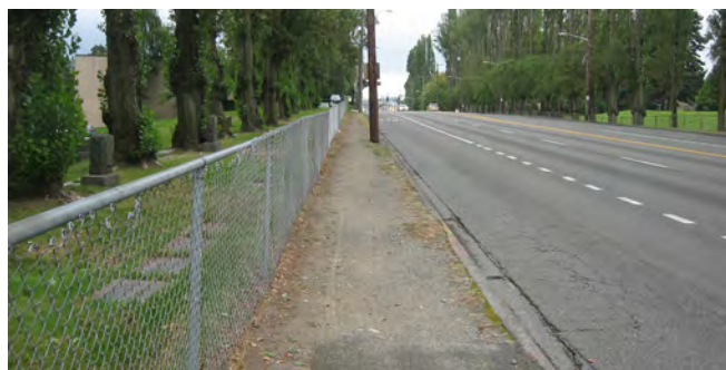
Separation from traffic is inadequate (the sidewalk is too close to the street).
