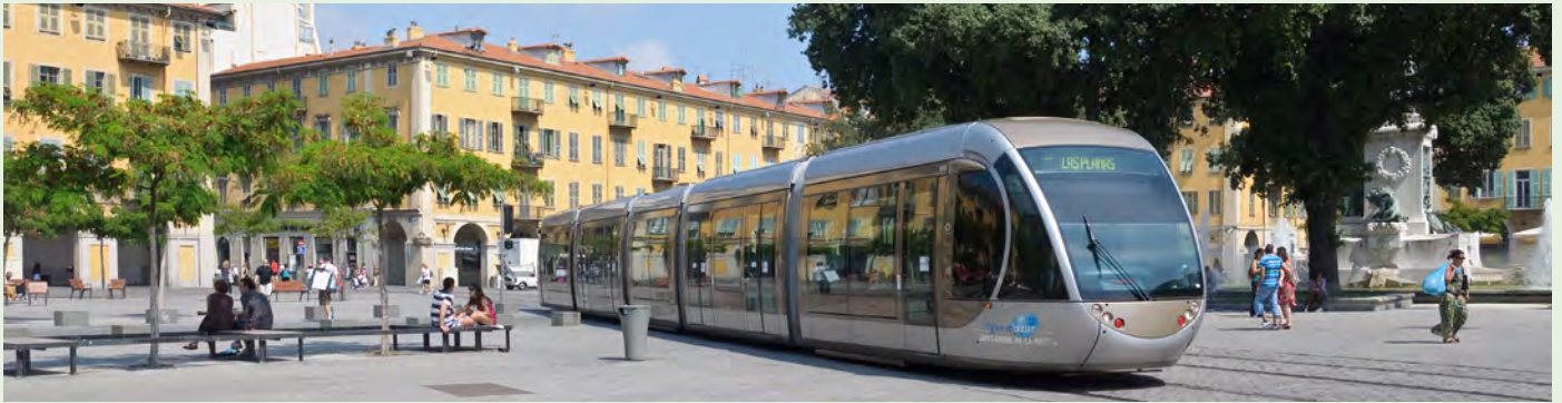
T1 tram in Nice's Place Giribaldi, where the tram runs without overhead wires, using batteries for a short section.
