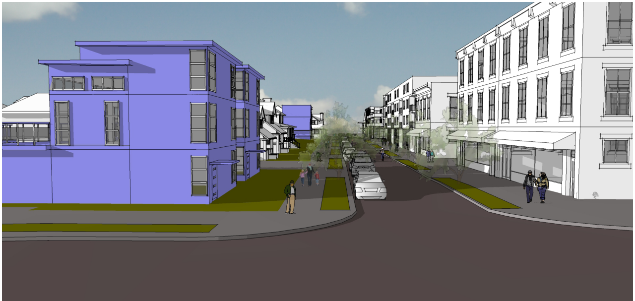
Existing context. Single-family zoned area (left side of street) and NC-40 zoned area (right side of street), provided for comparison. Buildings in blue illustrate the scale of single family home structures that could be built under existing regulations.
