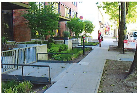
Street trees, swale and small patios provide a successful transition from public to private.
