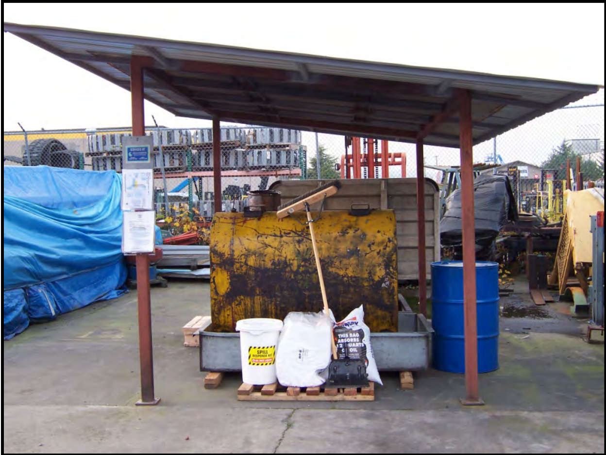
Figure 2. Waste Storage Area with Spill Kit and Posted Spill Plan.
