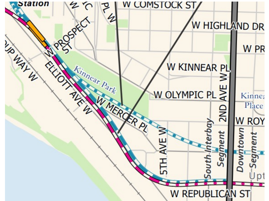
The “Elliott Snake” elevated guideway of SIB-1 and SIB-2 would cross Elliott Ave W three times in less than one mile. (Image: WSBLE DEIS Executive Summary)
