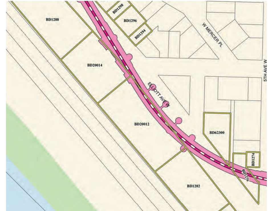
SIB-1 alternative in South Interbay would have numerous property and right-of-way impacts—including affected parcels on private property and column placements in Elliott Ave W. (Image: WSBLE DEIS. Appendix L)
