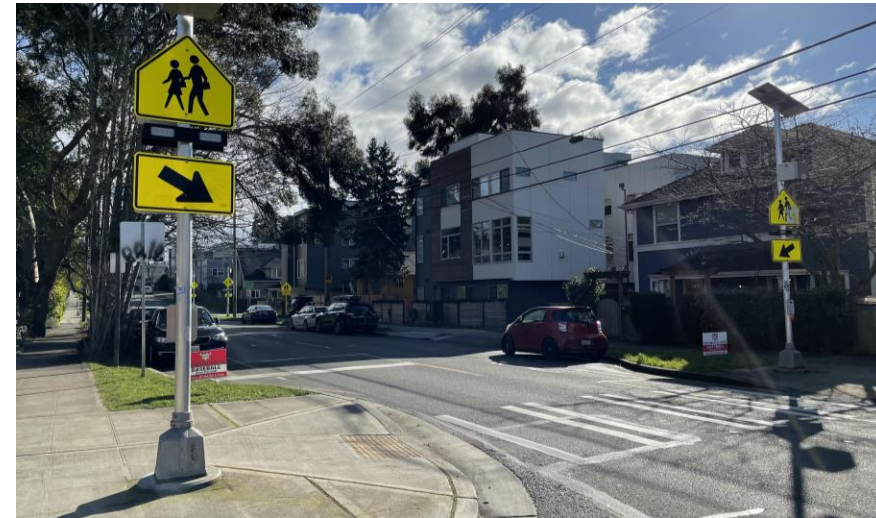
People crossing the street at Rainier Ave S and S Henderson St (top) A rectangular rapid flashing beacon at a marked crosswalk (bottom)
