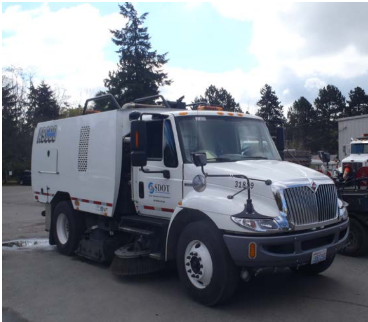
Figure 2-1. Schwarze model A9000 regenerative air sweeper
