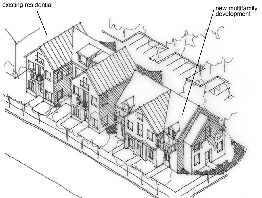
An example of massing, roof forms and elements such as dormers on new multifamily development to create scale compatibility with adjacent residential areas.
