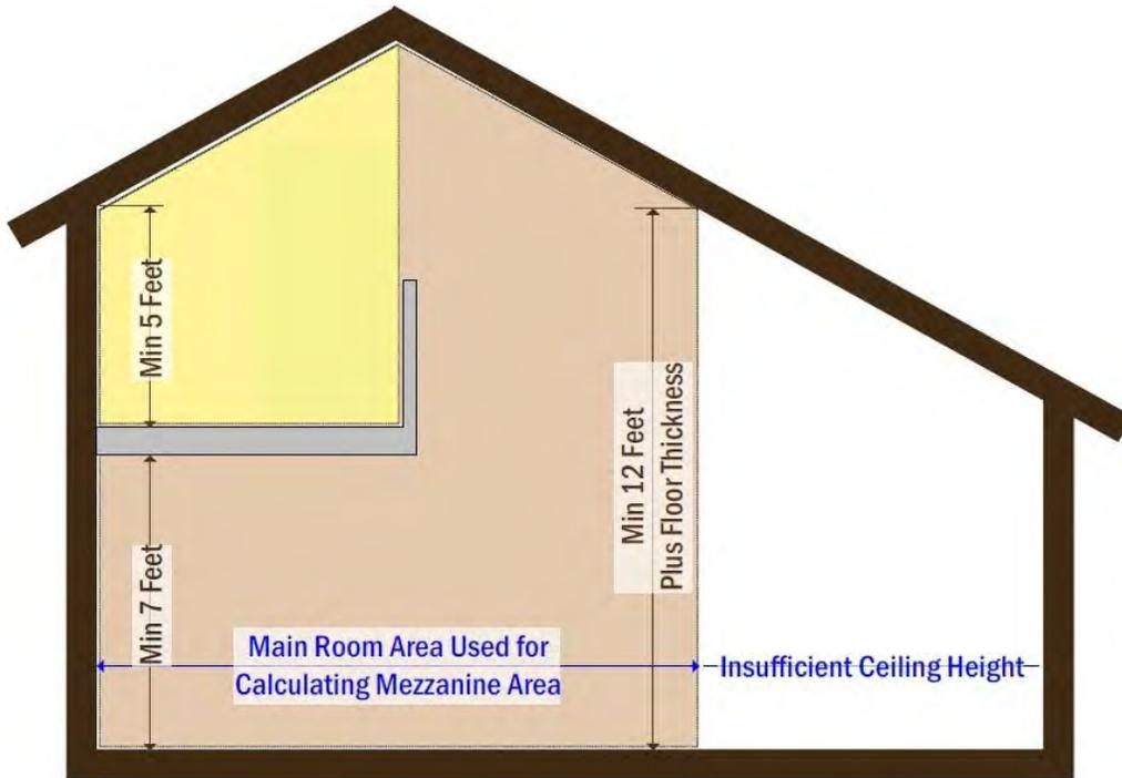
**Basis for Calculating Allowable Mezzanine Area
