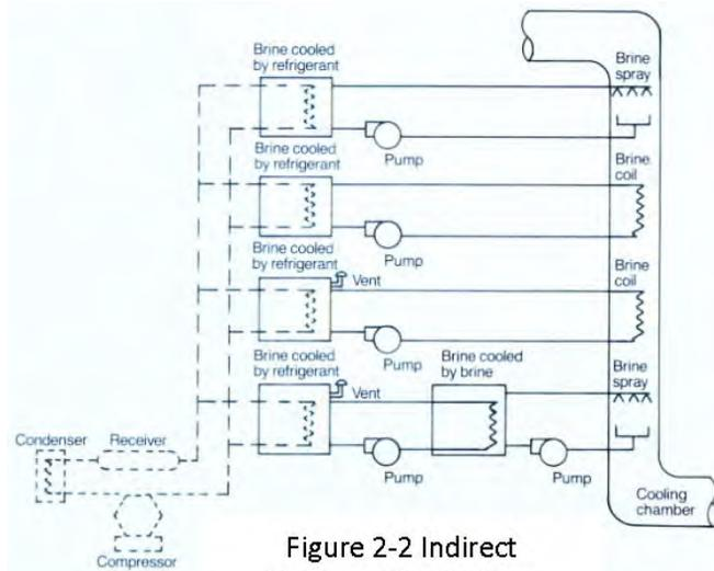
Figure 2-2 Indirect Refrigeration System
