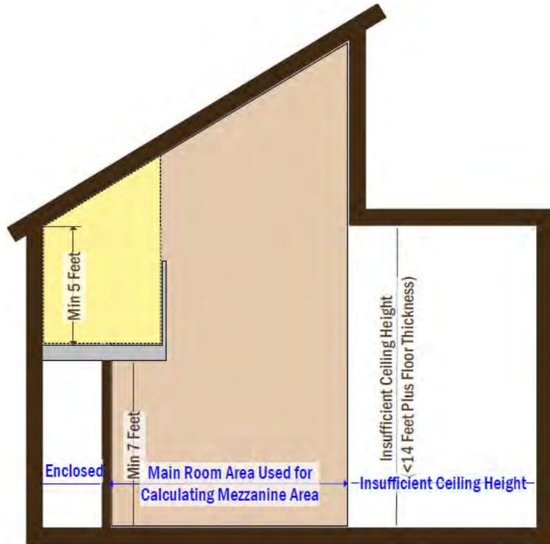
**Basis for Calculating Allowable Mezzanine Area
