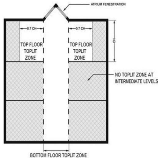
**C405.2.5.4 Atriums.** Daylight zones at atrium spaces shall be established at the top floor surrounding the atrium and at the floor of the atrium space, and not on intermediate floors, as indicated in Figure C405.2.5.4.
