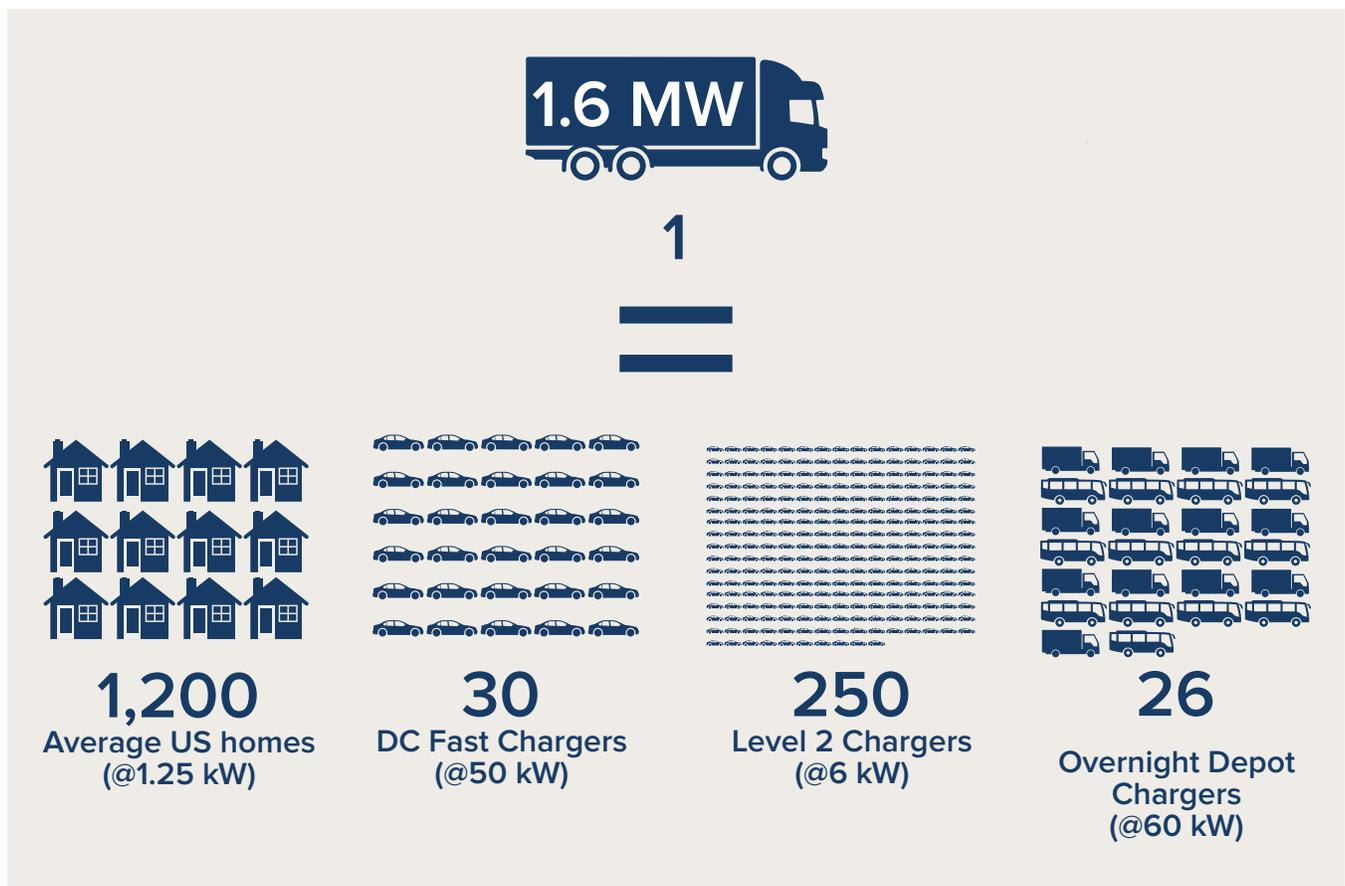
Electric trucks offer a double-edged sword in terms of their impact to the grid: they are likely to concentrate in industrial areas of cities making load planning simpler, but they draw significantly more power per charging event than POVs, potentially straining distribution grid capacity at those locations. If planned well, electric buses can improve grid asset utilization and present a new source of predictable revenue.
