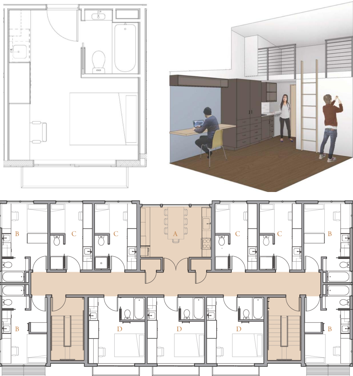
Figure 5: Yobi building visualization of loft space, and upper level floor plan. Credit Neiman Taber Architects.
