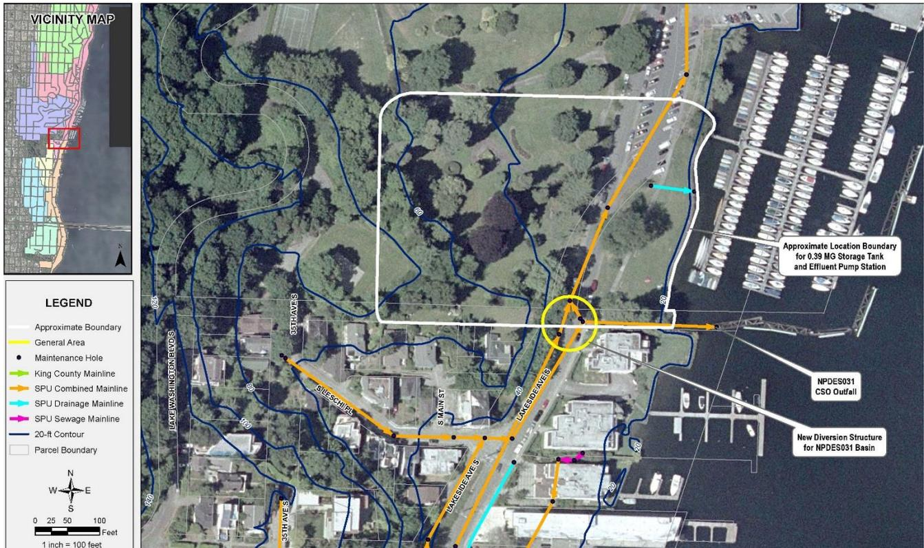
**Figure 5-23. CSO Outfall 031 and 032 Recommended Control Measure**
