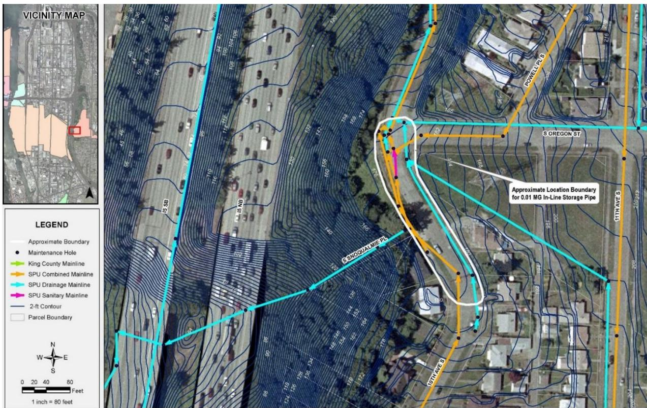
**Figure 5-12. Duwamish CSO Sub-basin 111H Recommended Control Measure**
