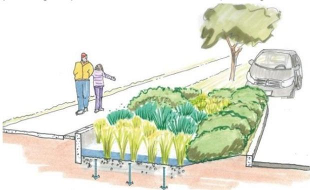
amount of stormwater reaching the City's combined sewer system by 6.5 MG each year and reduce the downstream storage control volume by 150,000 gallons. The project is also improving aesthetics, safety, and walking and biking mobility by overlapping with Seattle Department of Transportation's (SDOT's) proposed Neighborhood Greenway routes and community goals for improving the neighborhood.
