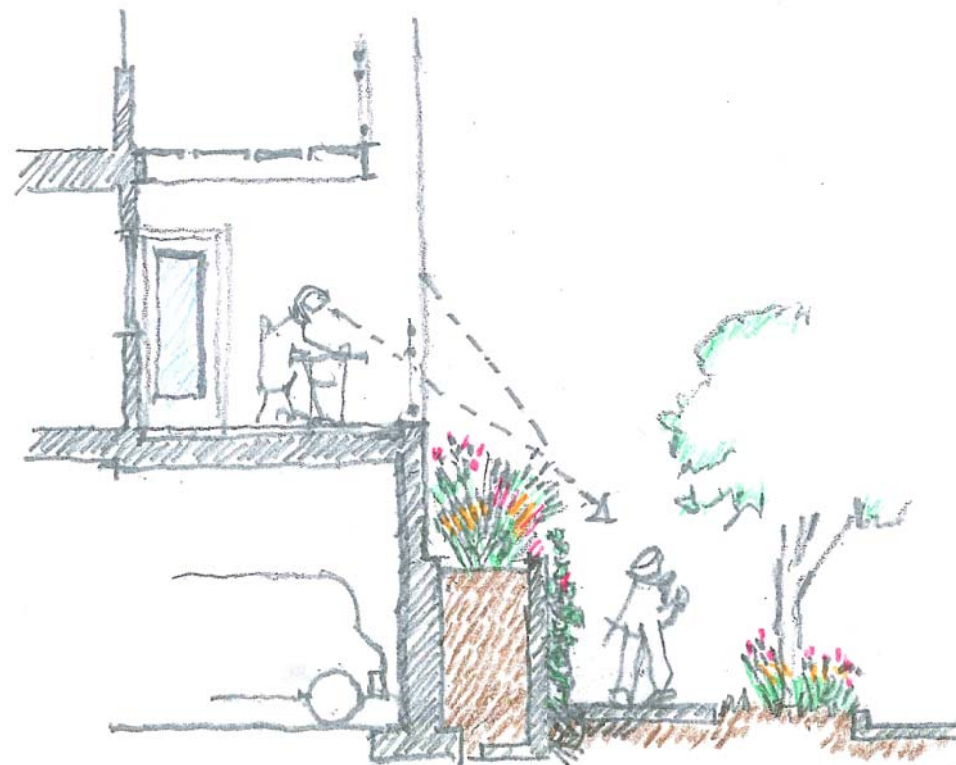
Retaining Wall Planter and GSI Between Buildings at Varying Heights Adjacent to Sidewalk
