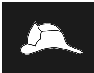
FIGURE 403.6.1.5.5 FIRE SERVICE ACCESS ELEVATOR SYMBOL
