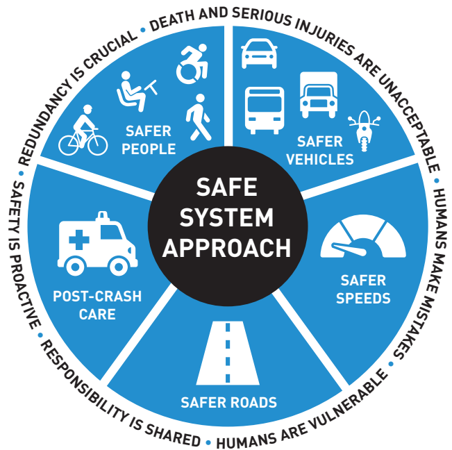
Figure 7. Six guiding principles and five elements of the Safe System Approach (credit: US Department of Transportation)
