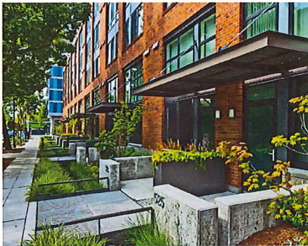
Residential uses at grade are set back from the sidewalk to provide transitional space and landscaping. The use of brick, awnings, and individual unit entries are engaging to passers-by.
