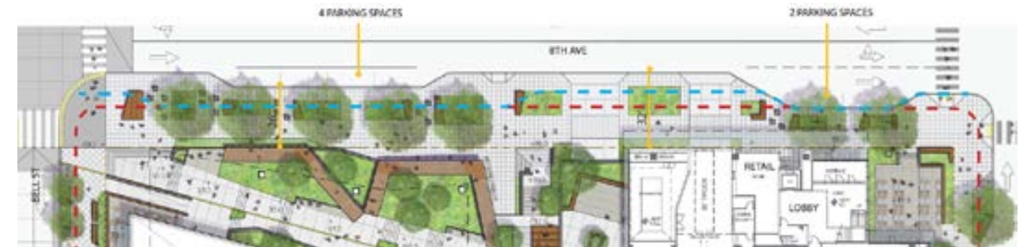
Figure 2. Revised curb line, previously proposed curb line (blue dashed line), and existing curb line (red dashed line) on 8th Ave.
