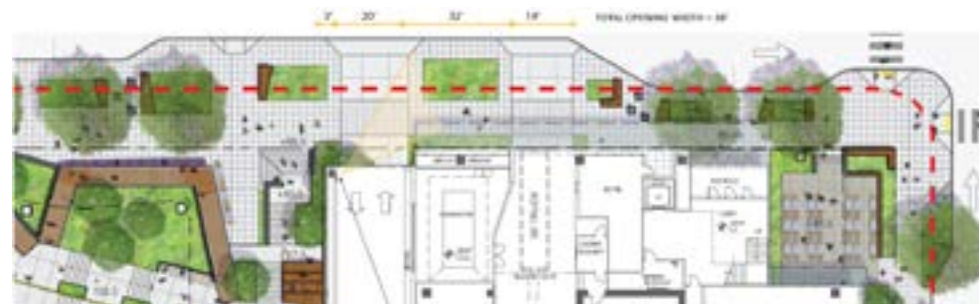
Figure 1. Updated plan for the 8th Ave streetscape, including narrower curb cuts for vehicle and loading access.
