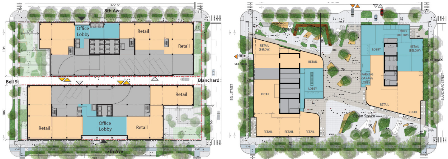
Figure 2. The no alley vacation (left) and full alley vacation (right) alternatives in plan view. Note that the vacation scheme includes an aerial connection between the two buildings at the third and fourth floors as illustrated by the dashed line.
