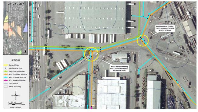
Figure 5-11. Duwamish CSO Sub-basin 111B and 111C Recommended Control Measure
