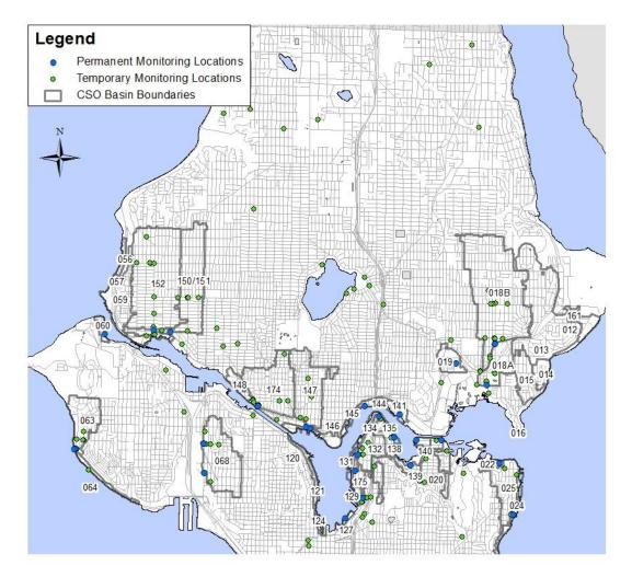
Figure 2-21. 2008-2010 Flow Monitoring Locations in Northern Seattle
