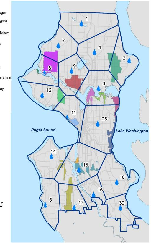
Figure 2-24. Thiessen Polygons for Each of the City's Rain Gauges
