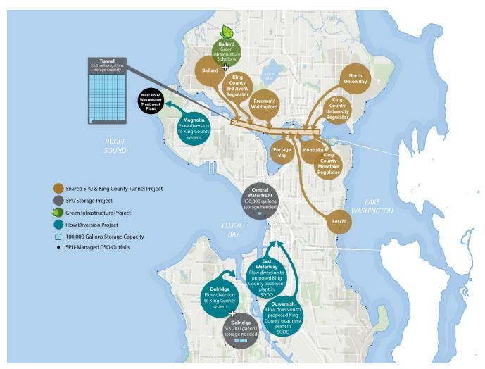
Figure 3-20. Shared Ship Canal Tunnel Option
