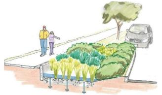
amount of stormwater reaching the City's combined sewer system by 6.5 MG each year and reduce the downstream storage control volume by 150,000 gallons. The project is also improving aesthetics, safety, and walking and biking mobility by overlapping with Seattle Department of Transportation's (SDOT's) proposed Neighborhood Greenway routes and community goals for improving the neighborhood.
