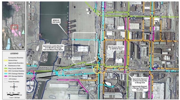
Figure 5-13. East Waterway CSO Outfall 107 Recommended Control Measure
