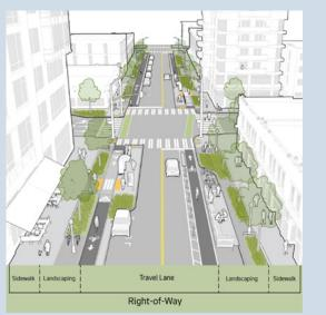
Figure 1: A representation of the Right-of-Way. Adapted from SDOT Streets Ilustrated.
