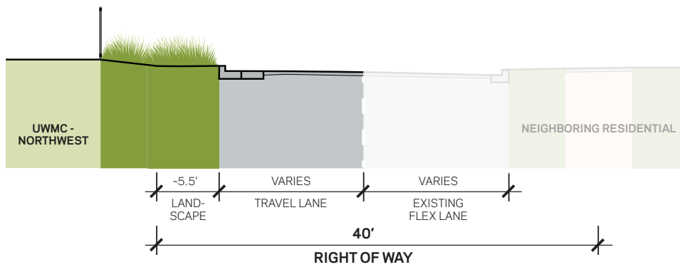
FIG 6.6 STREET SECTION AT BURKE AVE N - NORTHEAST CAMPUS EDGE
