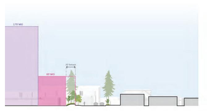
FIGURE 4.7 ALTERNATIVE 2 HEIGHT & SETBACK SECTION AT N120TH ST CAMPUS EDGE
