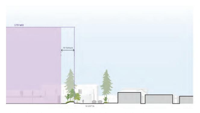
FIGURE 4.4 ALTERNATIVE 1 HEIGHT & SETBACK SECTION AT N120TH ST CAMPUS EDGE
