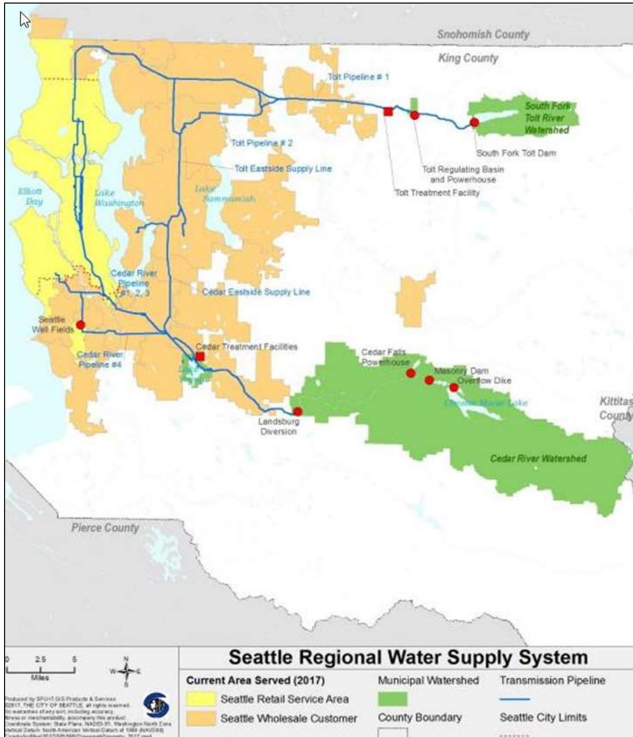
Figure A-169 Drinking Water Service Area, Facilities and Transmission Pipelines
